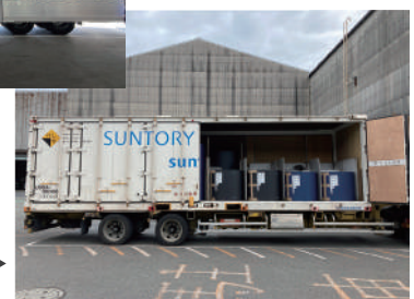
Example of loading in a 31-foot rail container
